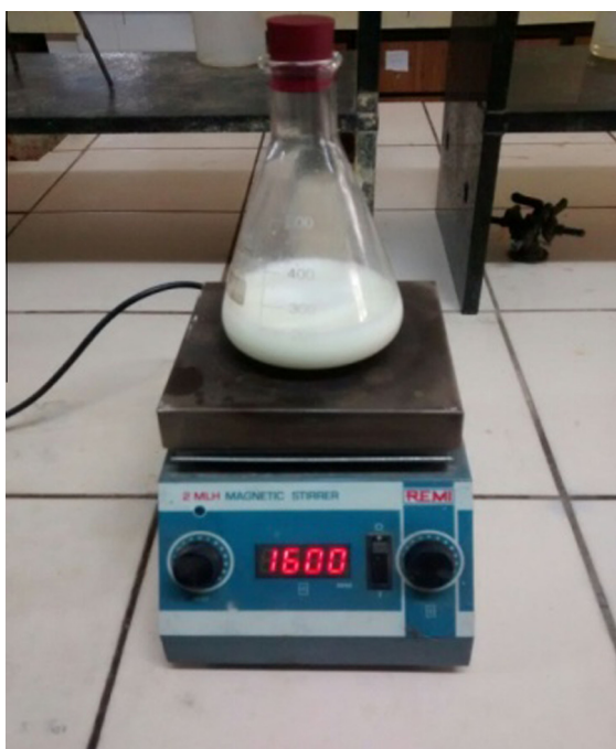
Figure 1 Magnetic stirrer setup.
