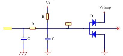
Figure 6. Clamp circuitry in sensor signal conditioning
