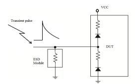
Figure 5. ESD Testing for DUT
