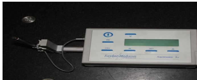
Figure 1. Taylor Hobson Surtronic 3+ machine
