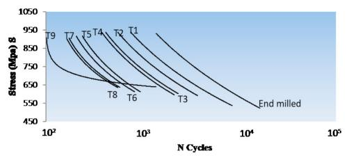
Fig. 9 S-N curve of SEDM samples compared with end milled
