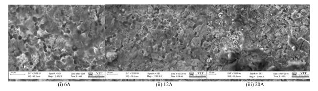
Fig. 6 SEM images of Inconel 718 after SEDM process.
