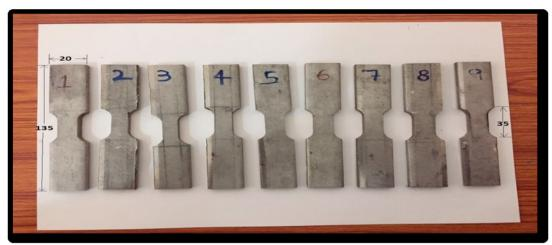
Fig. 5 ASTM E606 Fatigue Standard Samples.
