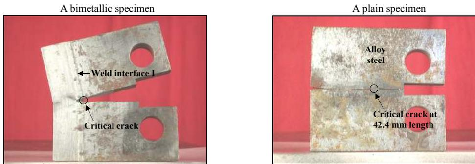
**Fig. 4 Fractured specimens**
