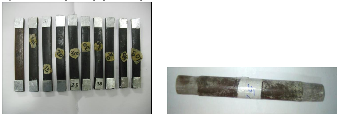
Fig. 1. Jute fibre (a) and Banana fibre (b) made hybrid polymer matrix composites at varying CNSL % prepared.
