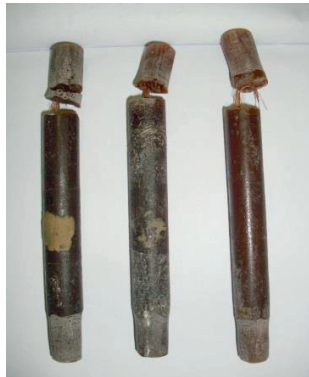
Fig. 4. Banana fibre composite after failure.
