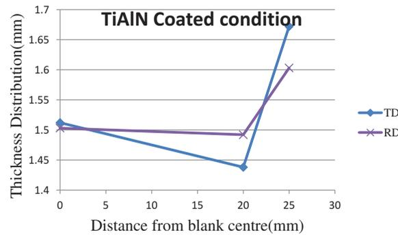
**Figure 4.** (a) Thickness variation under dry condition. (b) Thickness variation in oil-lubricated condition. (c) Thickness variation with TiAlN-coated condition.
