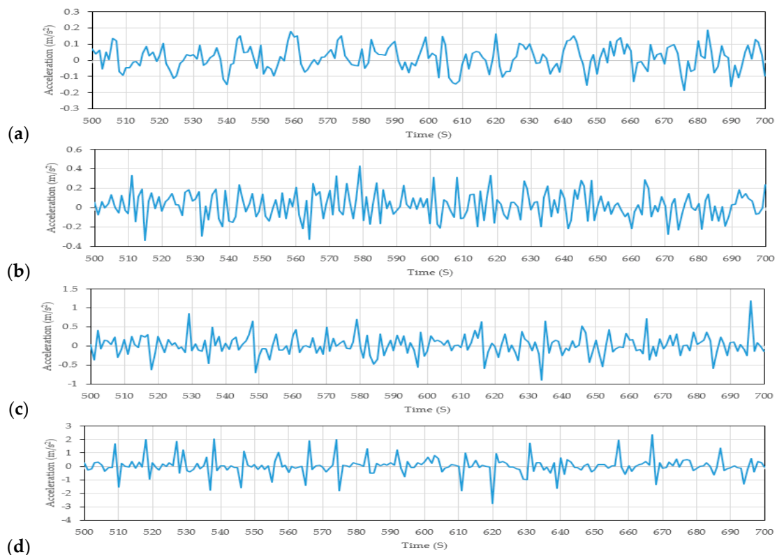
Figure 3. A closer view of acquired vibration signal for different bearing conditions. (a) No-Fault; (b) Inner Race Fault; (c) Outer Race Fault; (d) Ball Fault.
