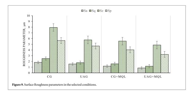
it combines the advantages of both techniques. The combination of MQL with UAG aids each other in lowering the forces while grinding.
