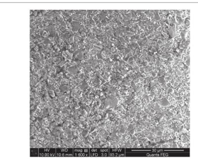
Figure 1. SEM image and of alumina sample as received.
