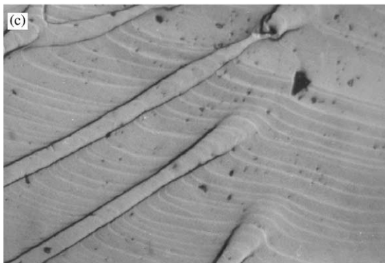
Fig. 2. Surface morphology of Co:BST single crystals: (a) vein-like structure, (b) layer growth pattern and (c) vein structure with two-dimensional growth.
