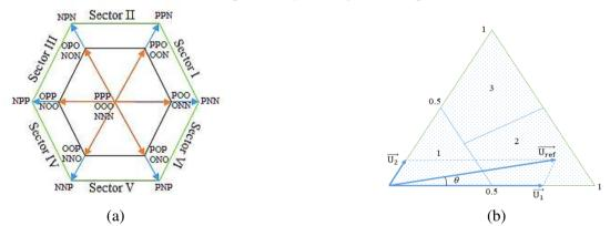
Figure 4. (a) SVM for 10 switch converter (b) Sector representation for normalized voltage vector
