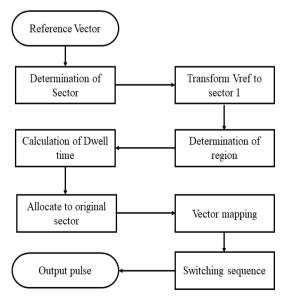
Figure 6. Flowchart for SVM calculation.
