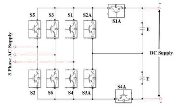
Figure 2. Circuit diagram for ILC.
