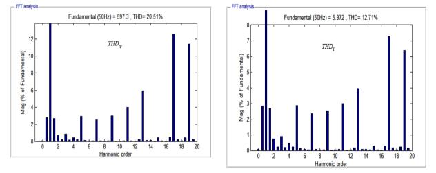
Figure 12. FFT Analysis for grid side output voltage and current for unbalanced condition.
