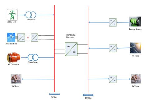
Figure 1. Diagrammatic Representation of Interlinking Converter for Bipolar Hybrid microgrid.
