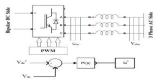
Figure 3. PWM control of ILC.
