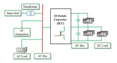
Figure 8. Block Diagram of MATLAB Simulation.
