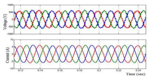
Figure 13. Simulated ac grid side output of Voltage and current for balanced condition.
