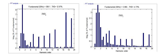
Figure 14. FFT Analysis for grid side output voltage and current for balanced condition.
