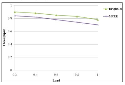
Figure 7 Throughput performance of DPQRS-M and MXRR under non-uniform bursty traffic using fanout splitting (see online version for colours)
