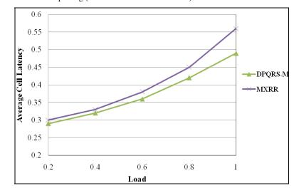
Figure 9 Average cell latency of DPQRS-M and MXRR under non-uniform bursty traffic using no fanout splitting (see online version for colours)
