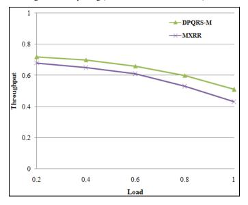
Figure 4 Throughput performance of DPQRS-M and MXRR under non-uniform unbalanced traffic using no fanout splitting (see online version for colours)
