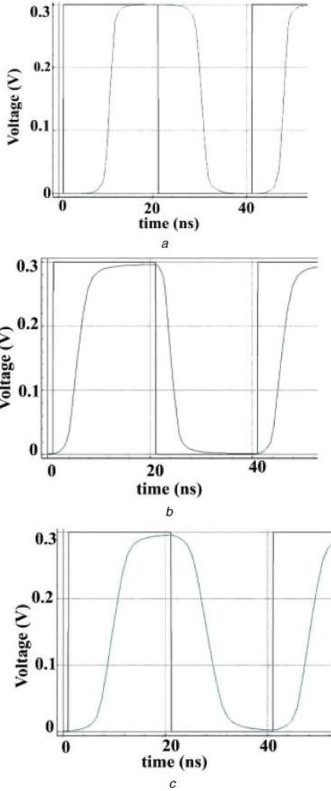
**Fig. 6** Input (maroon colour) and output (blue colour) waveforms of 500  $\mu\text{m}$ ,  $L_{ch} = 15 \text{ nm}$  for inverter and T-gate
