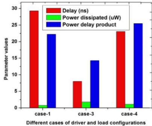
**Fig. 8** Comparison of parameters for cases 1, 3 and 4 for interconnect length of 500  $\mu\text{m}$
