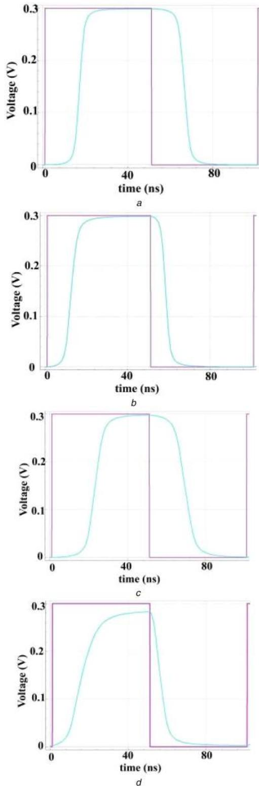
**Fig. 7** Input (maroon colour) and output (blue colour) waveforms of 1000  $\mu\text{m}$  long wires,  $L_{\text{ch}} = 15 \text{ nm}$
