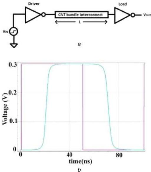
**Fig. 2** Inverter-wire-inverter model considered as case-1 in this paper (a) Driver-interconnect-load model, (b) Transient input and output waveform
