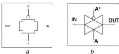
**Fig. 3** Transmission gate (a) Circuit connection, (b) Circuit symbol
