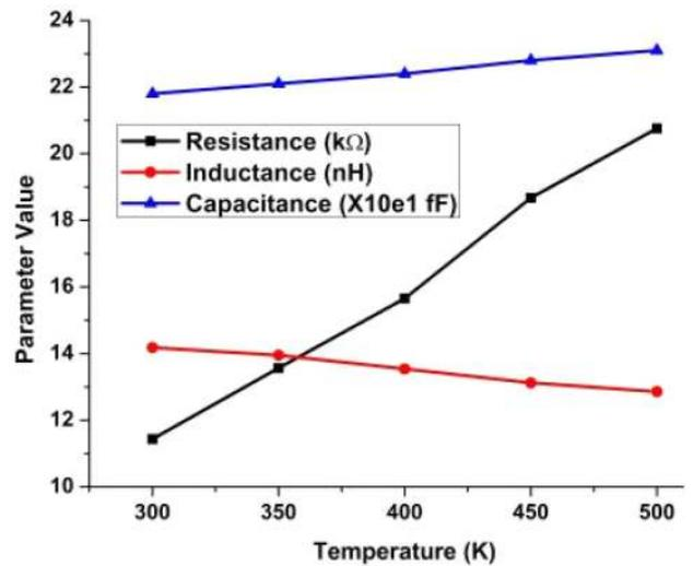
**Fig. 10** Resistance, inductance and capacitance vs. temperature
