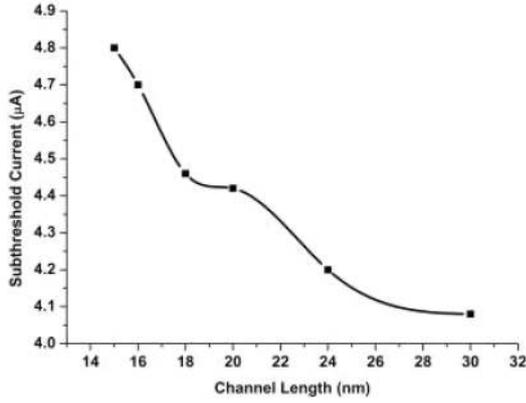
**Fig. 1** Sub-threshold current for different channel lengths of the CNTFETs in an inverter
