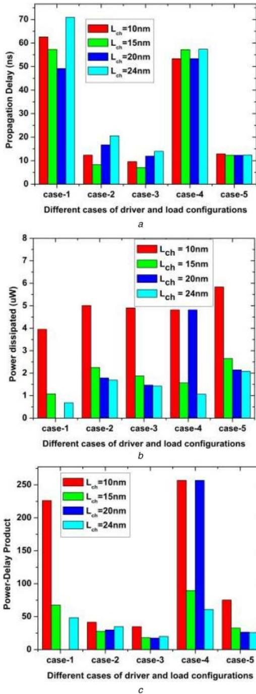
**Fig. 9** Output values for different cases as a function of different CNTFET channel lengths
