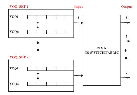
Figure 1: Input queued switch with virtual output queue
