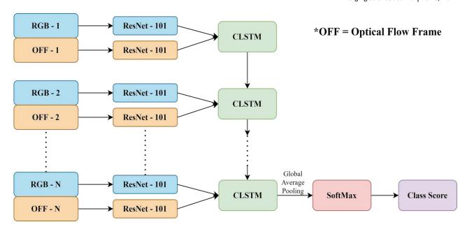
Figure 2. Basic proposed two-stream network architecture.
