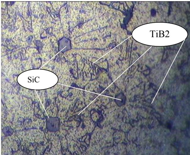
Fig. 1(c) Optical micrograph of (10SiC-5TiB<sub>2</sub>).
