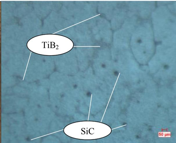
Fig.1(b) Optical micrograph of 10SiC-2.5TiB<sub>2</sub>
