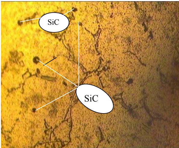
Fig.1(a) Optical micrograph of 10SiC-0TiB<sub>2</sub>
