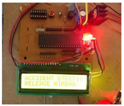
Figure 5. Interfacing Vibration Sensor with 8051.
