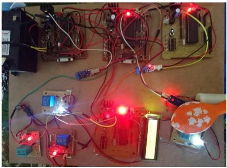
Figure 7. Airbag release system using fault tolerance concepts.
