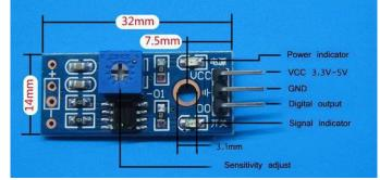
Figure 2. Pin diagram
