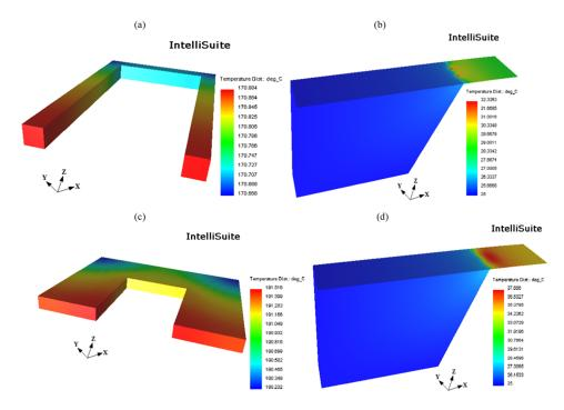
FIG. 6. For  $W_P = 5 \ \mu\text{m}$ : temperature profile (a) U-shaped piezoresistor operated in air, and (b) resistor integrated with the cantilever platform. For  $W_P = 25 \ \mu\text{m}$ : temperature profile (c) U-shaped piezoresistor operated in air, and (d) resistor integrated with the cantilever platform. In all the above simulations,  $L_P$  is fixed at 60  $\mu\text{m}$ .
