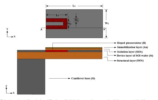
FIG. 1. A top view (without the immobilization and isolation layers) and a cross-sectional view (across AA') of the composite piezoresistive cantilever sensor with a diffused U-shaped piezoresistor. The symbols  $L_C$  and  $W_C$  represent the cantilever length and width respectively, whereas the symbols  $L_P$ ,  $W_P$ , and  $W_S$  depict the piezoresistor length, width and leg space respectively. This graphic is not drawn up to the scale.
