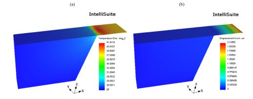
FIG. 7. Simulated (a) temperature and (b) displacement profiles of the cantilever platform with a U-shaped piezoresistor with the addition of the isolation layer.
