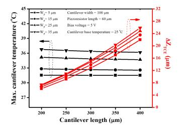
FIG. 9. Variation in the magnitude of maximum steady state cantilever temperature and TCE induced cantilever deflection versus the cantilever length for different piezoresistor width.
