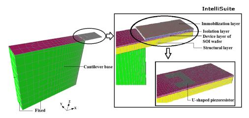
FIG. 2. A 3-D model of silicon dioxide piezoresistive cantilever sensor obtained using IntelliSuite<sup>®</sup> software. The graphic also contains zoom-in views of the constituent layers and the integrated U- shaped piezoresistor.
