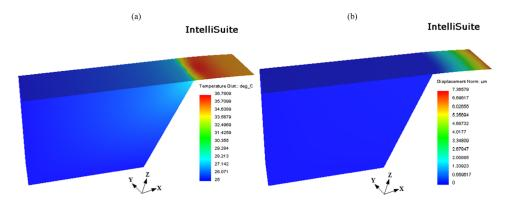
FIG. 8. Simulated (a) temperature and (b) displacement profiles of the cantilever platform with a U-shaped piezoresistor with the addition of both the isolation and immobilization layers.
