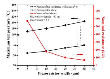
FIG. 5. Maximum cantilever temperature and nominal resistance as a function of the piezoresistor width.
