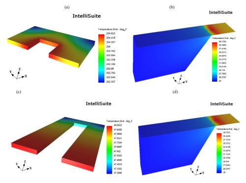
FIG. 4. For  $L_P = 60 \ \mu\text{m}$ : temperature profile (a) U-shaped piezoresistor operated in air, and (b) resistor integrated with the cantilever platform. For  $L_P = 180 \ \mu\text{m}$ : temperature profile (c) U-shaped piezoresistor operated in air, and (d) resistor integrated with the cantilever platform. In all the above simulations,  $W_P$  is fixed at 35  $\mu$ m.
