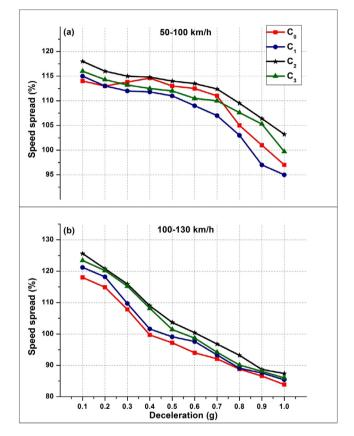
**Fig. 4.** Speed sensitivity of the friction composites at (a) mild condition (b) severe condition.
