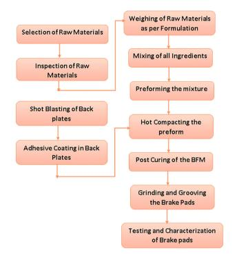
Fig.1. Manufacturing process flowchart.
