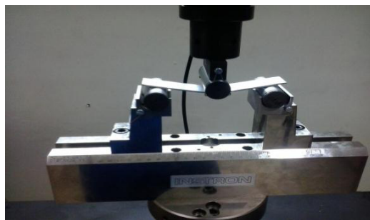
Figure 5. Three point bending with specimen
