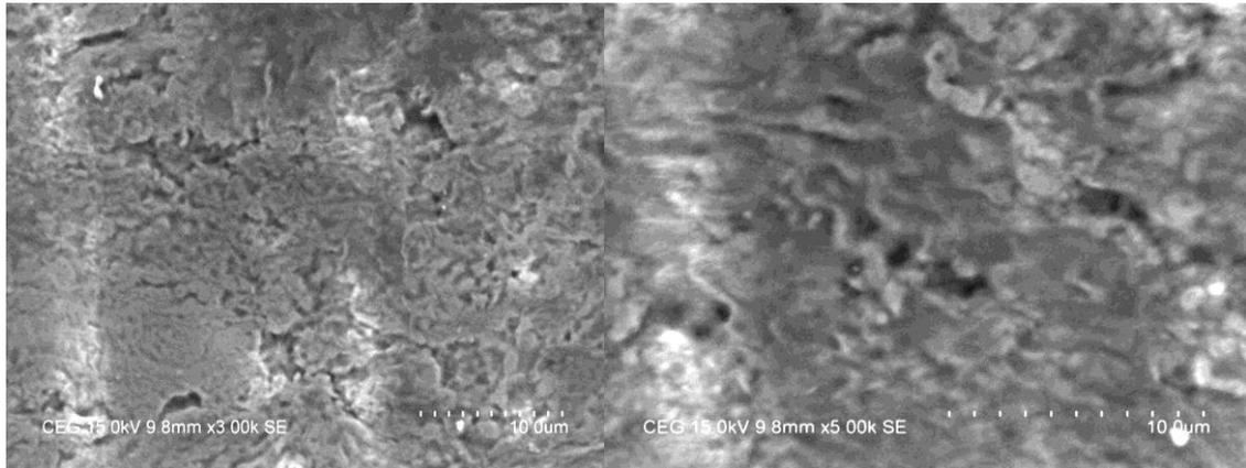
Fig. 6 SEM Image at the middle of the wear track 3000X and 5000X
