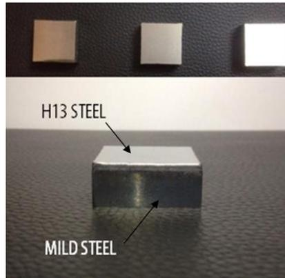
Fig.2. Photograph of Samples after coating
