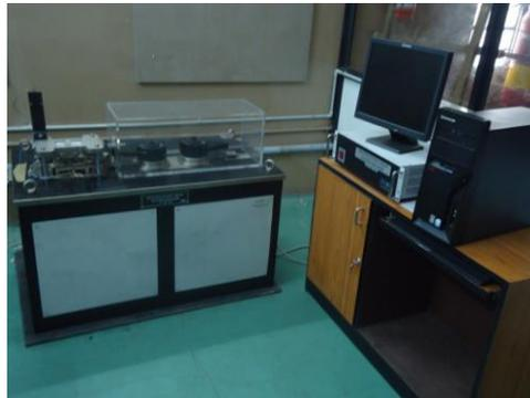
Fig. 3. Wear Testing Machine
