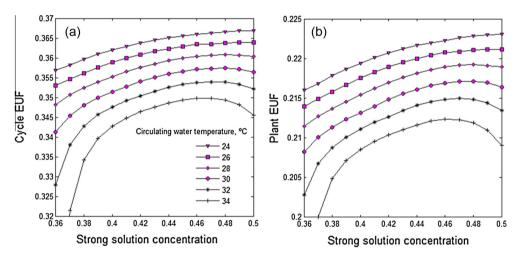
Figure 6 Influence of VAR's strong solution concentration with circulation water inlet temperature on (a) cycle EUF and (b) plant EUF.
