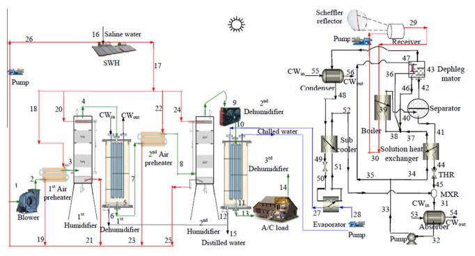
Figure 1 Two stage desalination with integrated VAR cooling.
