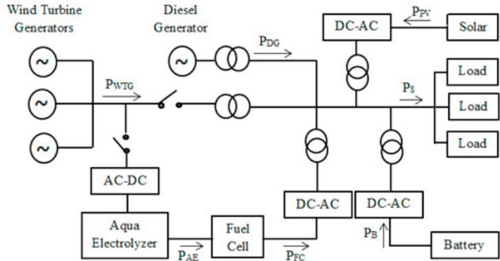
Fig. 1 System Configuration
