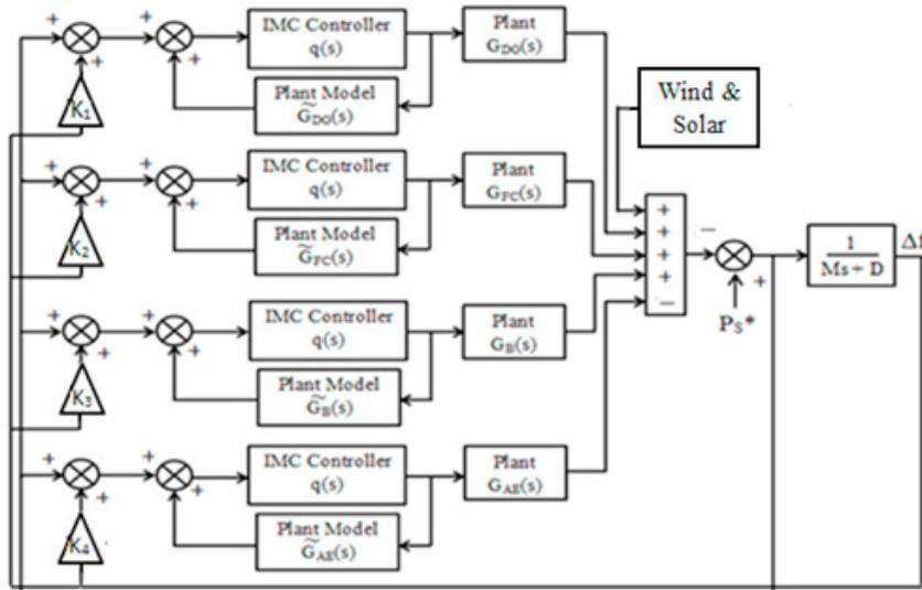
Fig. 2 Transfer function model of microgrid with IMC controller
