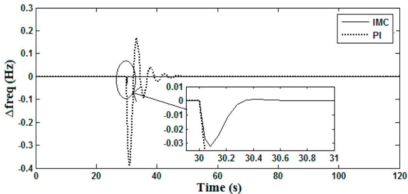
Fig. 4. (e) Frequency deviation of the microgrid system.
