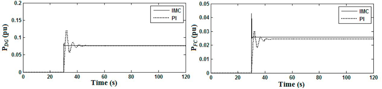
Fig. 5. (a) Power output of DG; (b) Power output of FC
