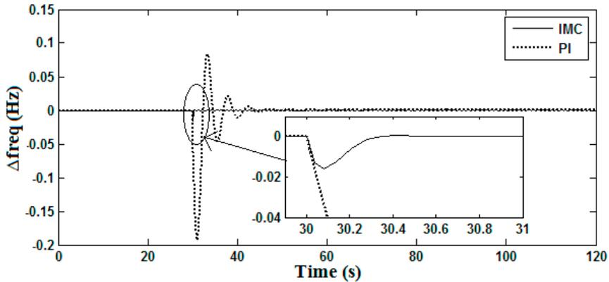
Fig. 5. (e) Frequency deviation of the microgrid
