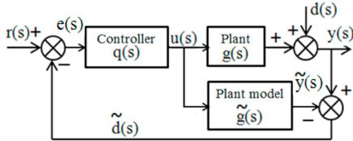
Fig. 3.(a) Structure of IMC
