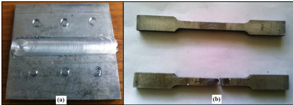
Fig. 8. Weld sample and tensile test specimen (a) FSW specimen; (b) Tensile test specimens
