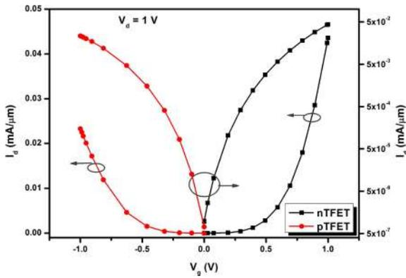
FIGURE 4.  $I_d$ - $V_g$  characteristics of n- and p-type DG TFETs.
