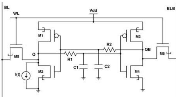
FIGURE 12. Radiation hardened 6T TFET SRAM cell.
