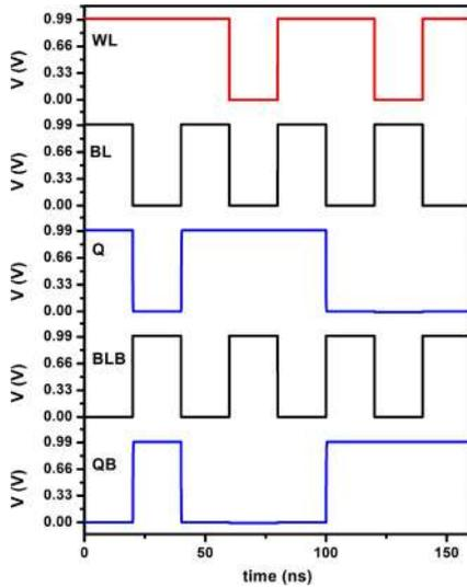
FIGURE 8. Timing diagram of 6T TFET SRAM.
