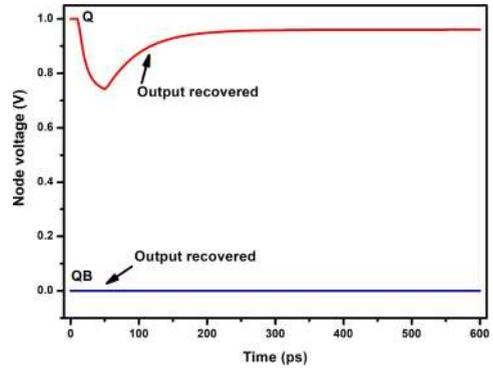
FIGURE 13. Node voltages of radiation hardened 6T TFET SRAM cell.
