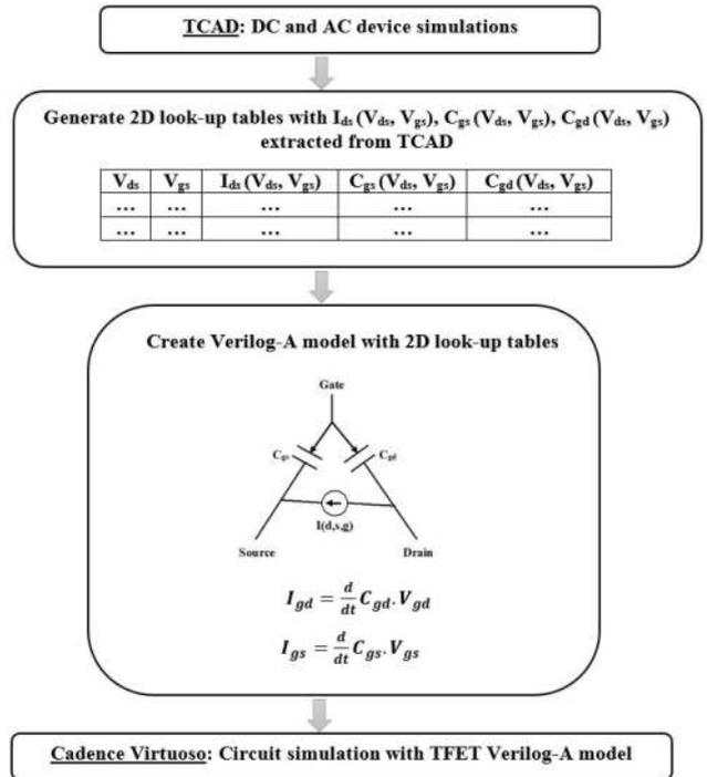
FIGURE 5. Flowchart for look-up table based Verilog-A model generation from TCAD simulations.
