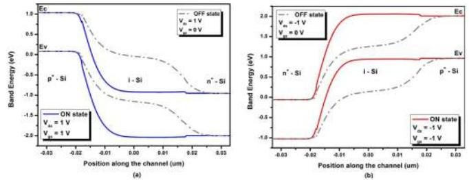
**FIGURE 3. Simulated energy band diagram (a) n-type DG TFET (b) p-type DG TFET.**
