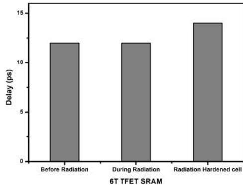
FIGURE 14. Delay of 6T TFET SRAM cell.
