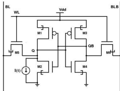
FIGURE 10. 6T TFET SRAM cell with injected current source.
