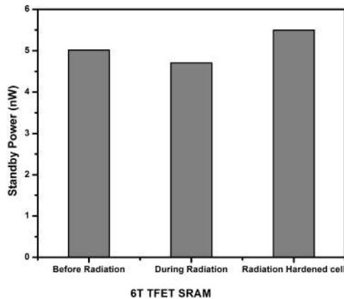
FIGURE 15. Standby power of 6T TFET SRAM cell.
