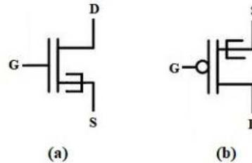
FIGURE 6. Symbol of DG TFETs (a) n-type (b) p-type.
