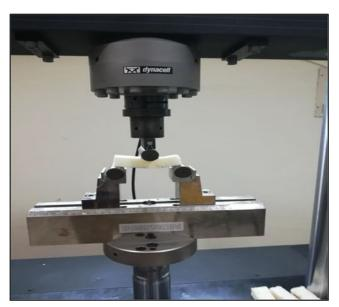
Figure 3. Flexural test specimen.
