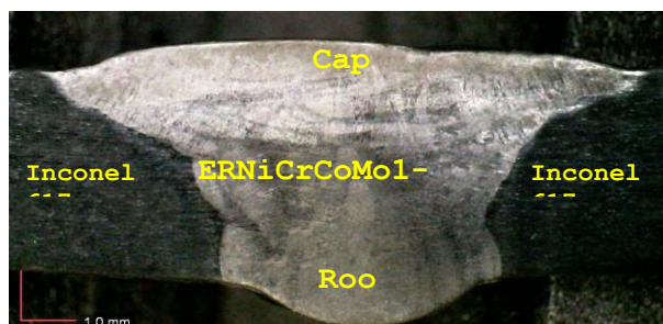
Figure 2. Macrostructure of Welded specimen using ERNiCrCoMo1
