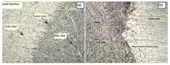
**Figure 4.** Weld interface region of joints fabricated with ER 309L (a) AISI 316 and (b) Duplex 2205
