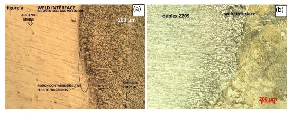
**Figure 3.** Weld interface region of joints fabricated with ER 316L (a) AISI 316 and (b) Duplex 2205
