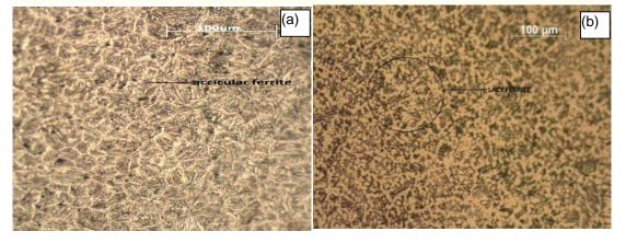
Figure 5. Fusion zone microstructure (a) ER 316L and (b) ER 309L
