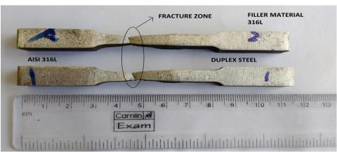
Figure 6. Tensile failure of weld joint fabricated with ER 316L filler wire
