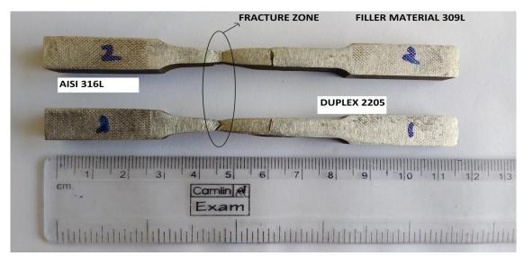
Figure 7. Tensile failure of weld joint fabricated with ER 309L filler wire
