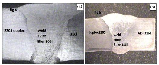
Figure 1. Marcograph of weld joints with (a) 316L filler wire (b) 309L filler wire
