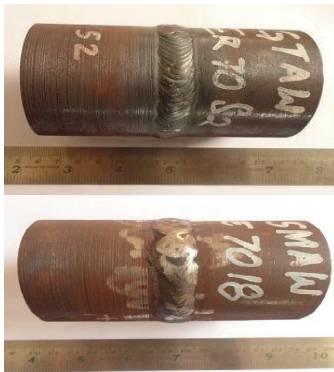
Fig.3 (a) Weldments of SA 210 C ferritic tubular steel using GTAW (top) and SMAW (b) Comparison of GTAW and SMAW tensile strengths
