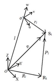
Figure 5: Single leg movement of 3-RPS Mechanism [2].
