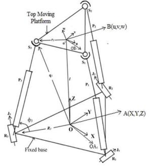
Figure 4: Schematic representation of Spatial 3-RPS [2].
