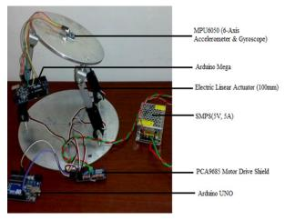
Figure 6: Experimental Prototype with Control system
