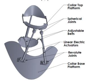
Figure 3: 3-RPS Rehabilitation Device.
