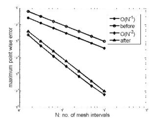
Fig. 3. Comparison of nodal errors on adaptive grid.
