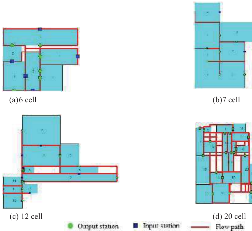
Fig. 8. The best layouts obtained by GA for the 4 test problems. a–d. W_1=0.5
