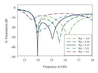
**Figure 6:** The S-parameters: variation in parameter " $W_p$ "
