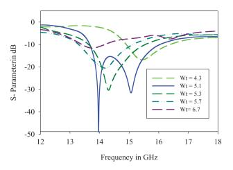
**Figure 8:** The S-parameters: variation in parameter " $W_t$ "
