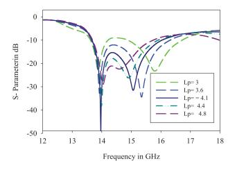
**Figure 5:** The S-parameters: variation in parameter " $L_p$ "
