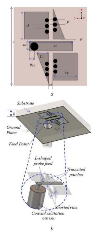
Figure 1: The antenna configuration. (a). The top view and (b) the perspective view
