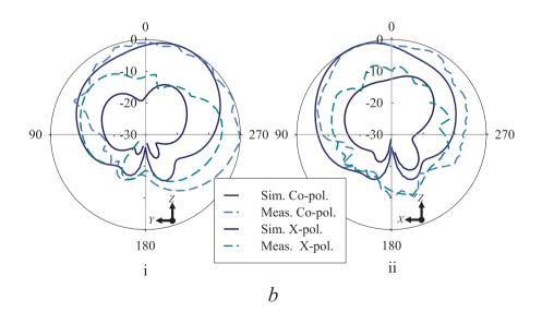
Figure 12: Radiation Profiles at: (a) 13.8 GHz: (i) yz-plane and (ii) xz-plane and (b) 15 GHz: (i) yz-plane and (ii) xz-plane.
