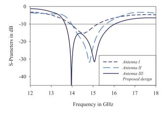
Figure 3: S-parameter response for design evolution
