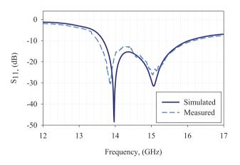
Figure 10: Simulated and measured reflection coefficients (S<sub>11</sub>)
