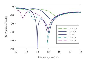
**Figure 7:** The *S*-parameters: variation in parameter " $L_t$ "
