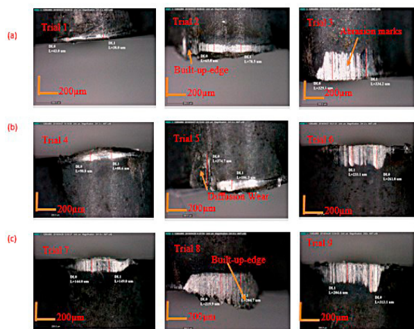
Fig. 8. Optical micrograph of tool wear image.
