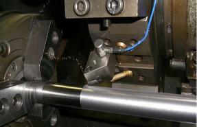
Fig. 1 Experimental setup showing the tool and accelerometer
