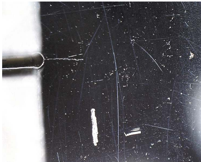
Fig. 3 Crack growth monitoring during fatigue precracking.
