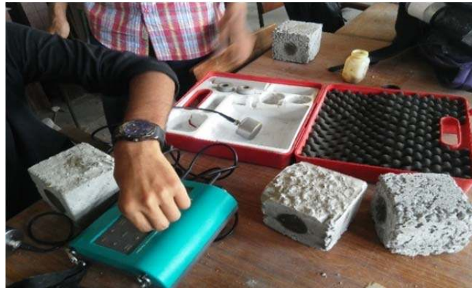
Fig. 5. UPV testing specimen
