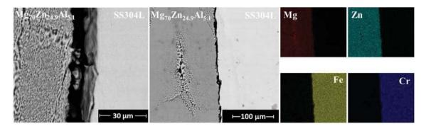
Fig. 4. The SEM images and corresponding EDX maps of the compatibility experiments between the  $Mg_{70}Zn_{24.9}Al_{5.1}$  eutectic alloy and the 304L stainless steel containment material.
