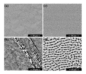
Fig. 2. SEM images of Mg70Zn24.9Al5.1 (a,b) and Zn85.8Al8.2Mg6 (c,d) eutectic alloys.
