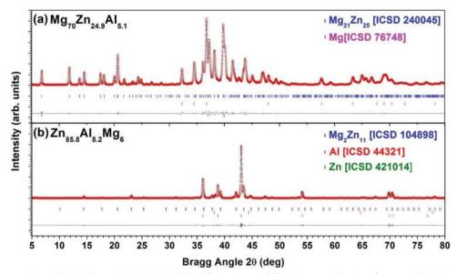
Fig. 1. Experimental (red cricles, oo) and calculated (black line, --) X-ray diffraction patterns for the refinements of (a) the  $Mg_{70}Zn_{24.9}Al_{5.1}$  and (b) the  $Zn_{85.8}Al_{8.2}Mg_6$  alloys. The bars in the lower part of the graphics represent the Bragg peak positions that correspond to the identified phases.
