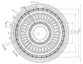
All Dimensions are in mm Fig 1: CAD Drawing of Analytical Plate topview with it's dimensions
