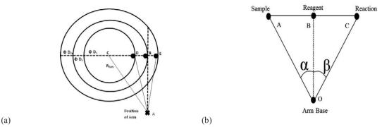
Fig.3. (a) Position with the analytical plate and (b) Triangle formed by the sampling and reagent arm motion over the batch analyzer
