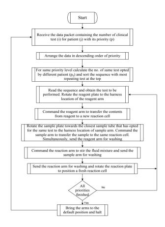
Fig 5. Flowchart for Random Access Algorithm implemented in Sampling and Reagent Arm with analytical plate
