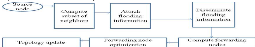
Fig 4. Functional Architecture for flooding scheme
