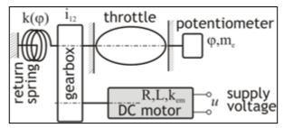
Figure 1. Schematic Diagram of an Electronic Throttle Control [17]
