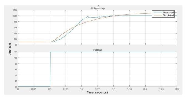
Figure 10. Percentage of Throttle Opening and Step input v/s Time plotted in MATLAB for ETB (Model using single nonlinearity)
