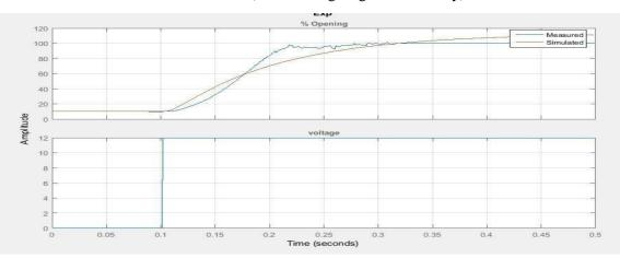
Figure 11. Throttle Opening and Step input v/s Time plotted in MATLAB for ETB (Model using two nonlinearity)
