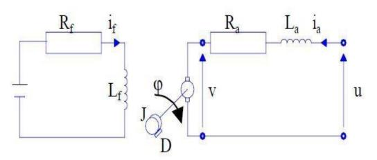
Figure 3. Linear Model for Electronic Throttle Control [16]
