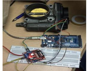
Figure 2. Experimental Setup for Electronic Throttle Control
