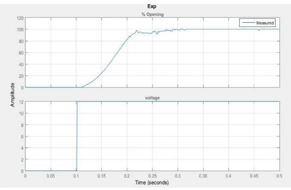
**Figure 7.** Percentage of Throttle Opening and Step input v/s Time plotted in MATLAB for ETB (Linear Condition)
