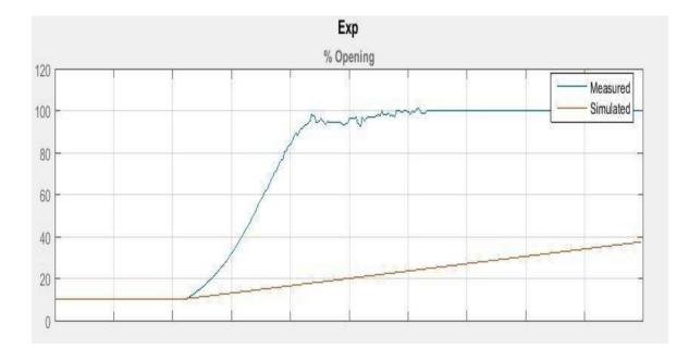
**Figure 8.** Percentage of Throttle Opening and Step input v/s Time plotted in MATLAB for ETB (Linear Model)
