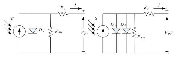
Fig.1. Single diode model
