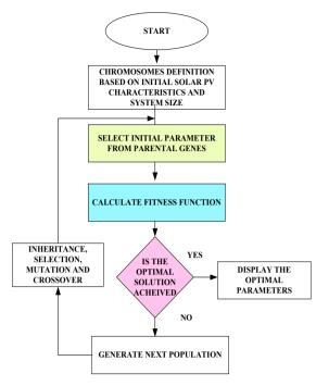
Fig.4.Flowchart for Genetic Algorithm
