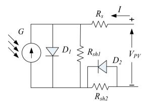
Fig.3. Reverse double diode model
