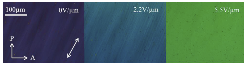
FIG. 8. The textures are recorded by POM under crossed polarizers on a planar-aligned cell of thickness 9\ \mu\text{m} filled with DR133 at a temperature of (T_{AC} + 1)\ ^\circ\text{C} in the \text{SmA}^* phase for different strengths of the applied electric field. T_{AC} is the \text{SmA}^* to \text{SmC}^* transition temperature. The double headed arrow represents the rubbing direction in the cell. A large increase in the field-induced birefringence is recorded as typical texture for de Vries Smectic.
