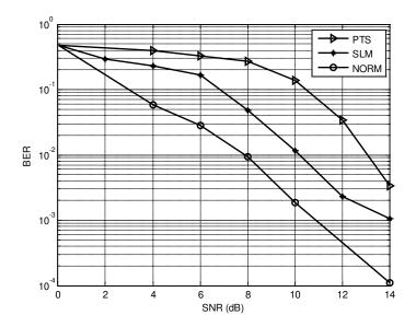
Figure 8 BER performance of NORM, PTS and SLM.
