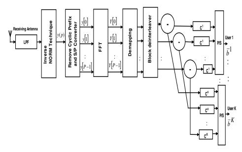
Figure 3 MC-CDMA receiver with inverse NORM technique.
