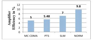
Figure 7 Amplifier efficiency analysis of NORM compared with PTS, SLM and conventional technique without PAPR reduction.
