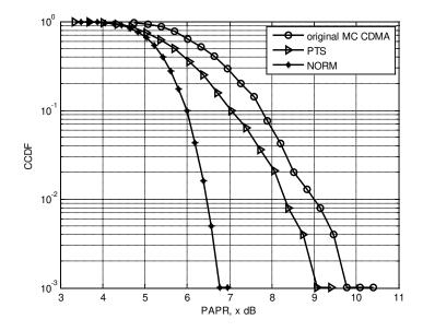
**Figure 4** CCDF performance of NORM technique with PTS and conventional technique without PAPR reduction in MC CDMA system.
