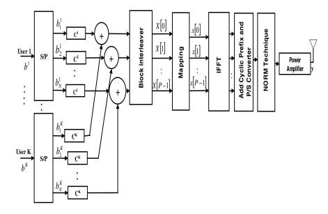
Figure 1 MC-CDMA transmitter with NORM technique.
