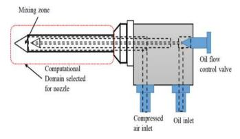
Fig 1. Schematic of nozzle used for the MQL.
