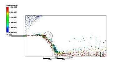
(e) Velocity contour for 200 ml/h flow rate
