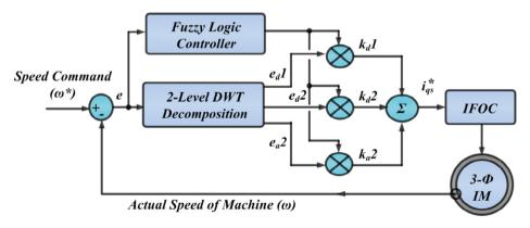
Fig. 1. Schematic of the proposed wavelet-fuzzy based speed compensator for IFOC IM drive.
