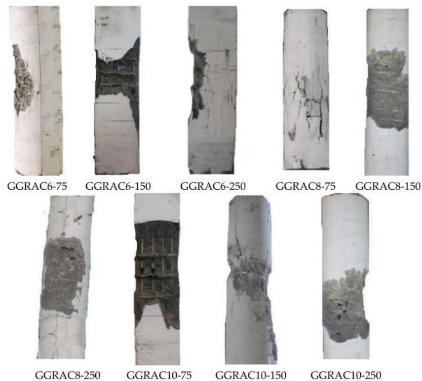
**Figure 5.** Crack initiation of GGRAC compressive members.
