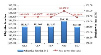
Figure 4 Comparison of proposed approach with other methods for 34-bus system at full load.
