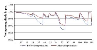
Figure 7 Comparison of voltage profile of 118-bus system at full load.
