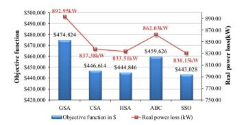
**Figure 8** Comparison of proposed approach with other methods for 118-bus system at full load.
