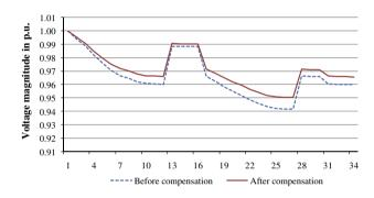
Figure 3 Comparison of voltage profile of 34-bus system at full load.
