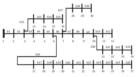
Figure 2 Single line diagram of 34-bus system.
