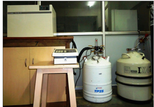
Figure 2. PLANER Kryo 560-16 cryogenic freezer.
