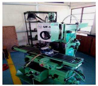
Fig. 3 Knee-type vertical milling machine
